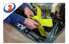
A. If the radiator is fitted, remove the top hose, slacken the mountings screws on both sides of the radiator and gently pivot the radiator forward.
