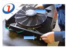
A. Fit the fan assembly to the radiator by slotting it into position.
