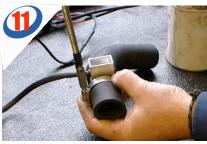
A. Fit both pieces of hose to the EFC ensuring the open top of the EFC points in the correct direction for access to the white slot when adjusting later. B. Fit both hose clips, ensuring they are accesible from above.
